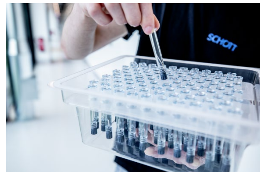
An employee holds a prefillable polymer syringe above a nest and tub.
