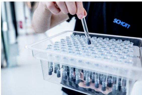
An employee holds a prefillable polymer syringe above a nest and tub. Image: SCHOTT Pharma/Oana Szekely
